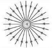
Fig 9.6: The electric field lines are directed radially inward towards a negative-point charge -q.
