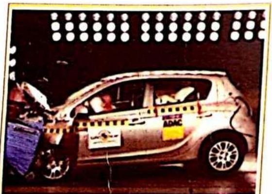
The crumple zone is designed to absorb energy from a collision and reduce the force of collision. Folding during a crash increases the impact time. Time to come to halt is increased so the force is decreased.
