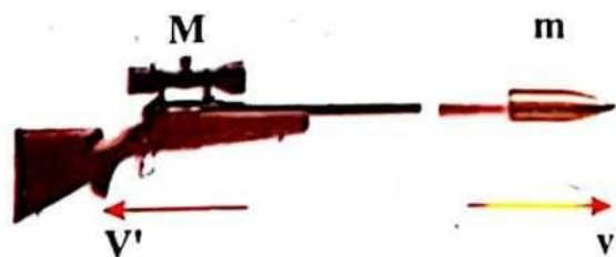
Fig.3.31: Conservation of momentum in firing a gun
