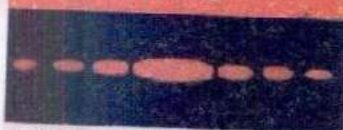
Diffraction pattern of a single human hair under laser beam illumination.
