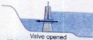
High tide: Water is allowed to flow back into the basin, driving turbines.
