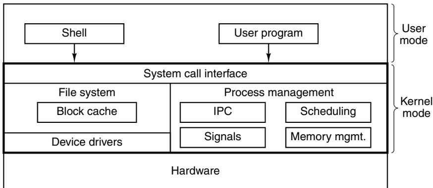
**Figure 6-30.** The structure of a typical UNIX system.
