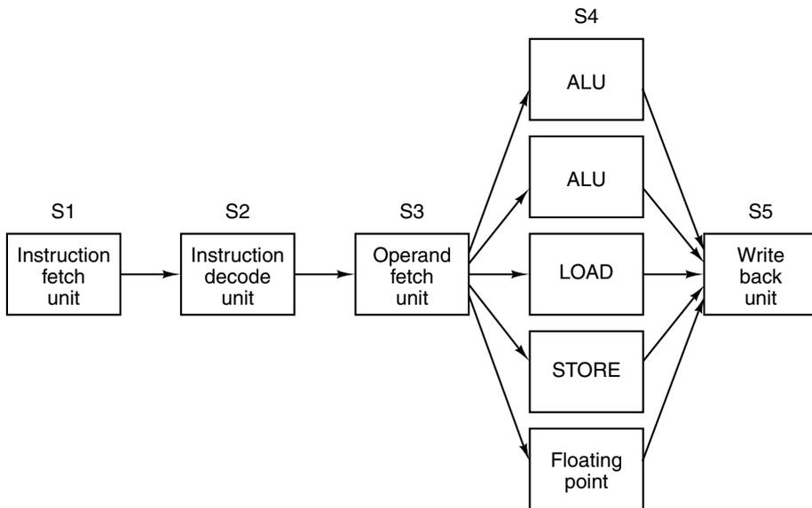
**Figure 2-6.** A superscalar processor with five functional units.
