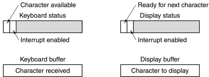
**Figure 5-31.** Device registers for a simple terminal.
