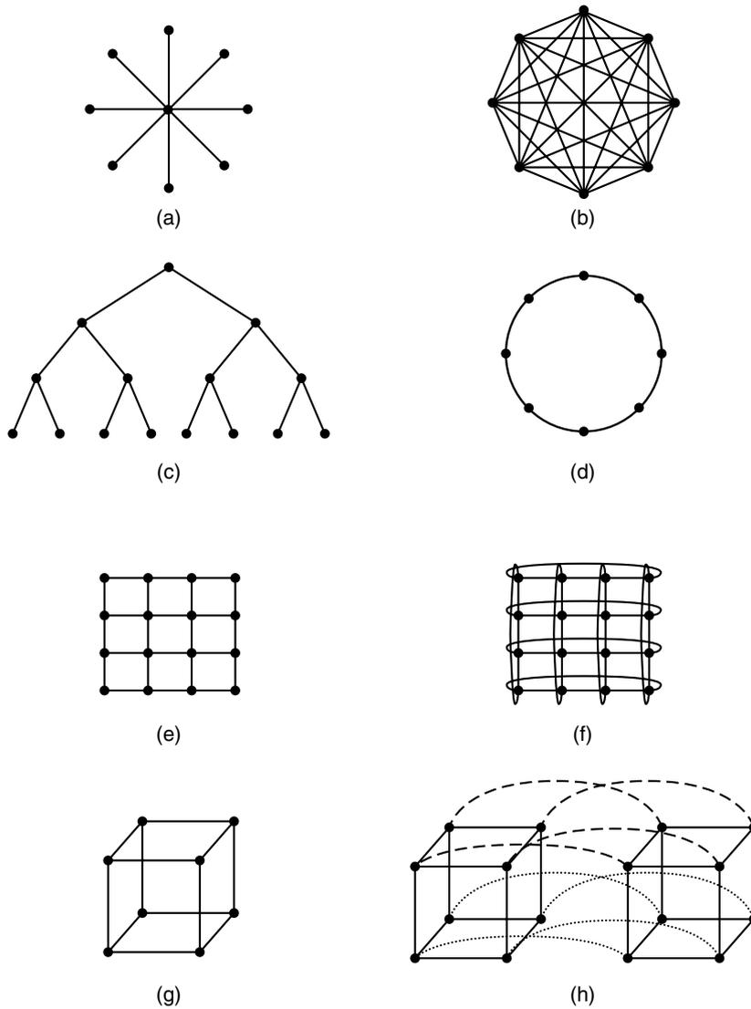
**Figure 8-35.** Various topologies. The heavy dots represent switches. The CPUs and memories are not shown. (a) A star. (b) A complete interconnect. (c) A tree. (d) A ring. (e) A grid. (f) A double torus. (g) A cube. (h) A 4D hypercube.
