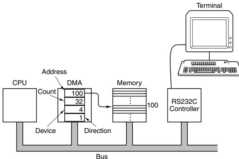
**Figure 5-33.** A system with a DMA controller.
