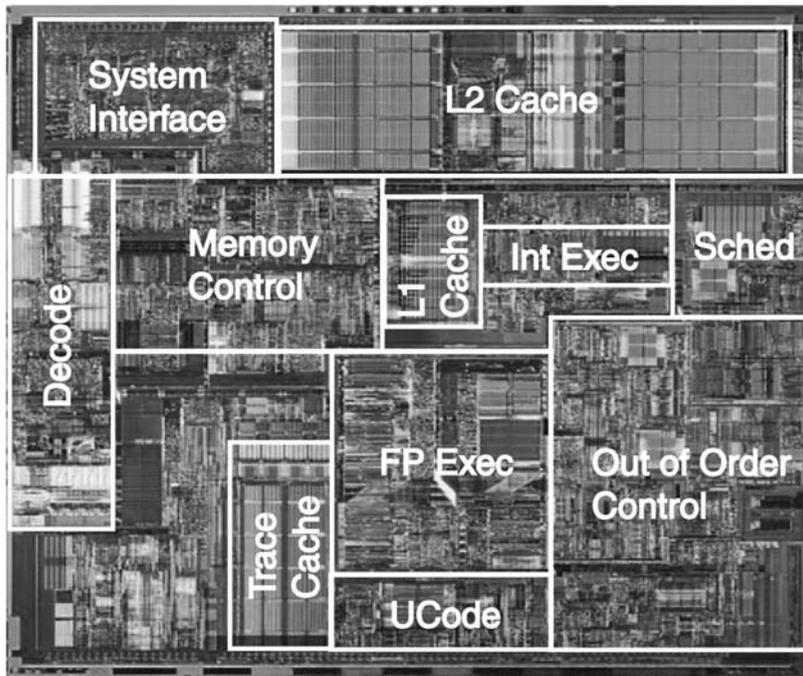
**Figure 1-12.** The Pentium 4 chip. The photograph is copyrighted by the Intel Corporation, 2003 and used by permission.
