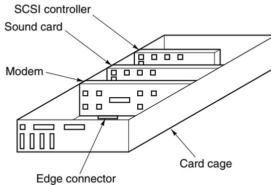
**Figure 2-28.** Physical structure of a personal computer.
