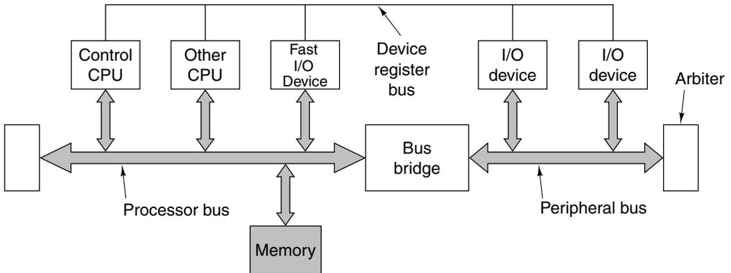
**Figure 8-12.** An example of the IBM CoreConnect architecture.
