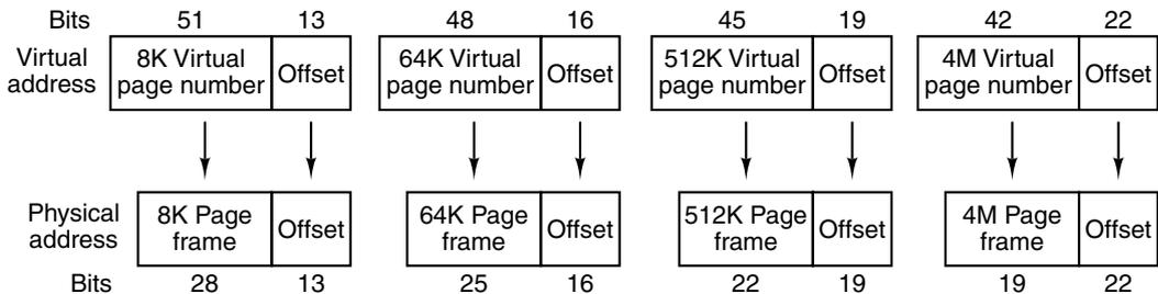
Figure 6-17. Virtual to physical mappings on the UltraSPARC.
