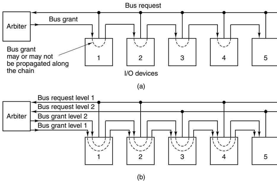
**Figure 3-40.** (a) A centralized one-level bus arbiter using daisy chaining.
