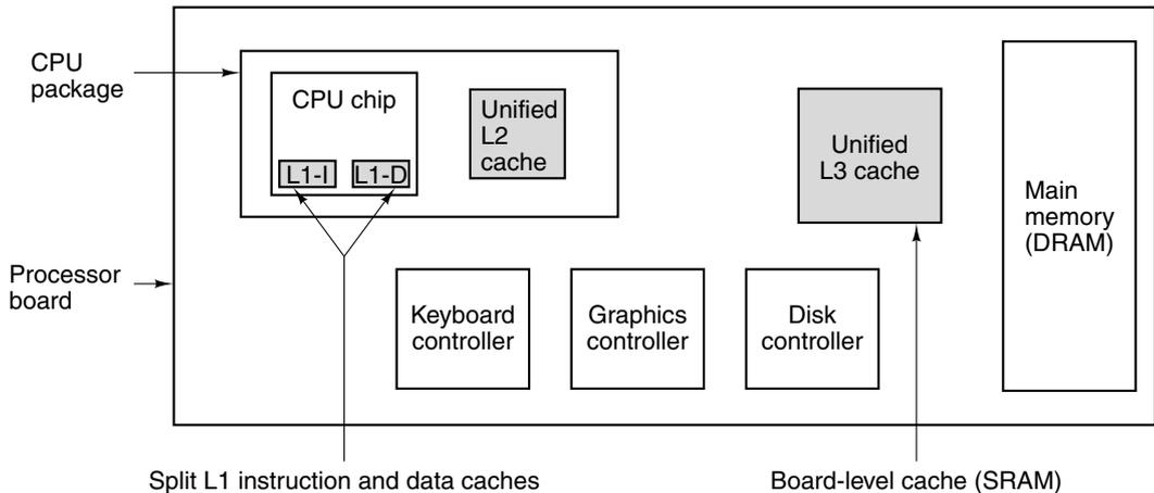
**Figure 4-37.** A system with three levels of cache.
