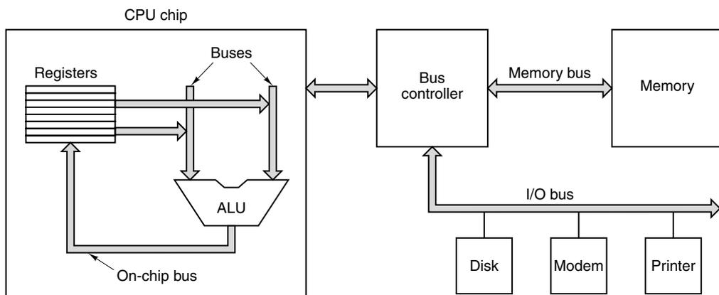
**Figure 3-35.** A computer system with multiple buses.
