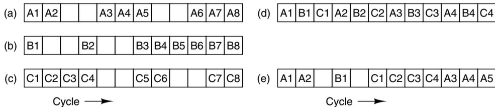
**Figure 8-7.** (a)–(c) Three threads. The empty boxes indicated that the thread has stalled waiting for memory. (d) Fine-grained multithreading. (e) Coarse-grained multithreading.
