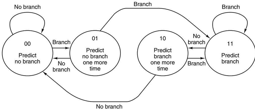
**Figure 4-42.** A 2-bit finite-state machine for branch prediction.
