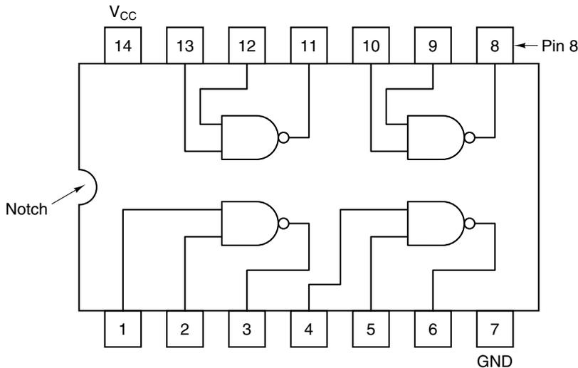
**Figure 3-10.** An SSI chip containing four gates.
