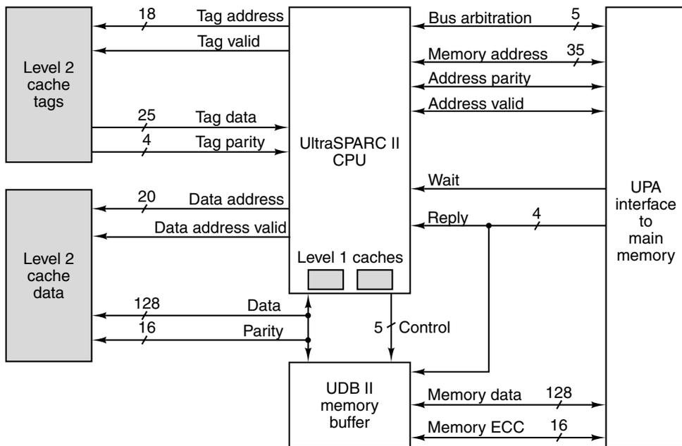
**Figure 3-48.** The main features of the core of an UltraSPARC III system.
