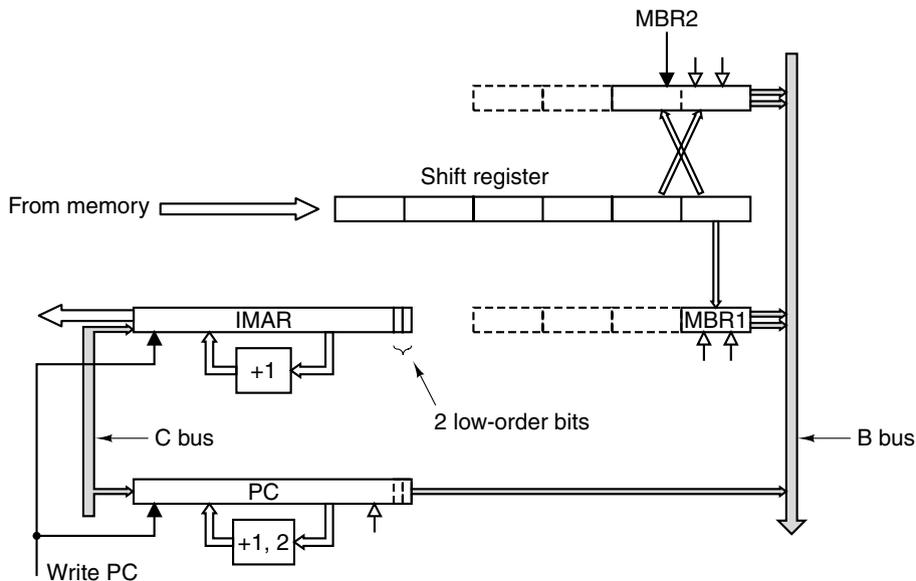
**Figure 4-27.** A fetch unit for the Mic-1.
