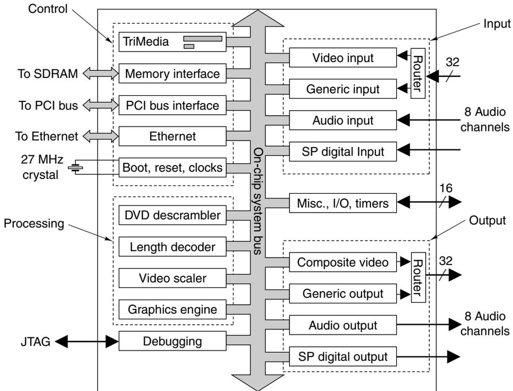
**Figure 8-16.** The Nexperia heterogeneous multiprocessor on a chip.
