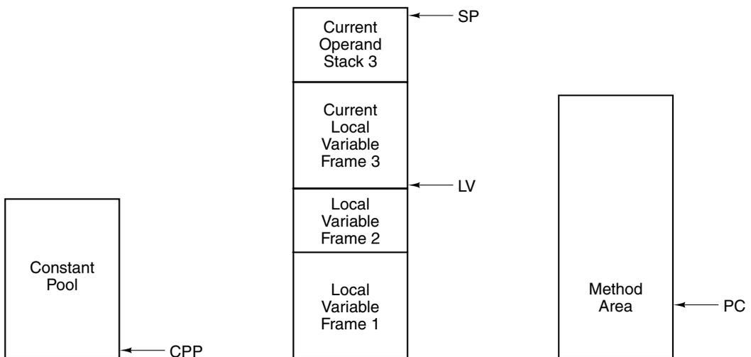
**Figure 4-10.** The various parts of the IJVM memory.
