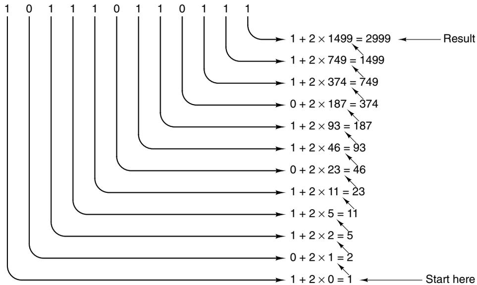
**Figure A-6.** Conversion of the binary number 10110110111 to decimal by successive doubling, starting at the bottom. Each line is formed by doubling the one below it and adding the corresponding bit. For example, 749 is twice 374 plus the 1 bit on the same line as 749.
