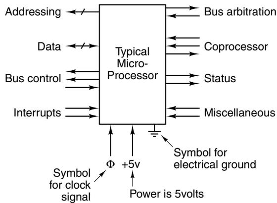
**Figure 3-34.** The logical pinout of a generic CPU. The arrows indicate input signals and output signals. The short diagonal lines indicate that multiple pins are used. For a specific CPU, a number will be given to tell how many.
