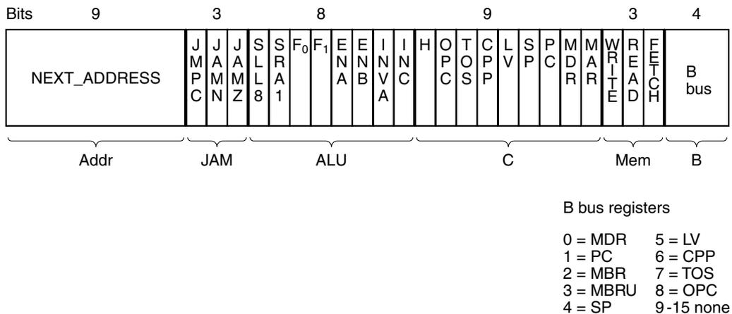
**Figure 4-5.** The microinstruction format for the Mic-1.
