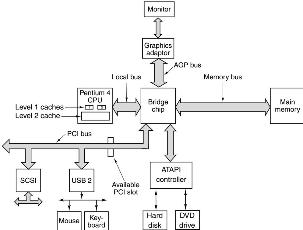
**Figure 3-53.** The bus structure of a modern Pentium 4.
