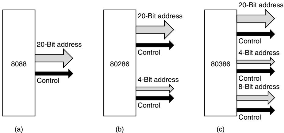
**Figure 3-37.** Growth of an address bus over time.
