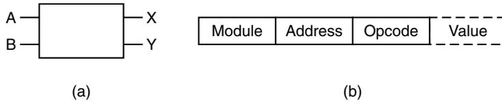
**Figure 8-28.** (a) A 2 × 2 switch. (b) A message format.
