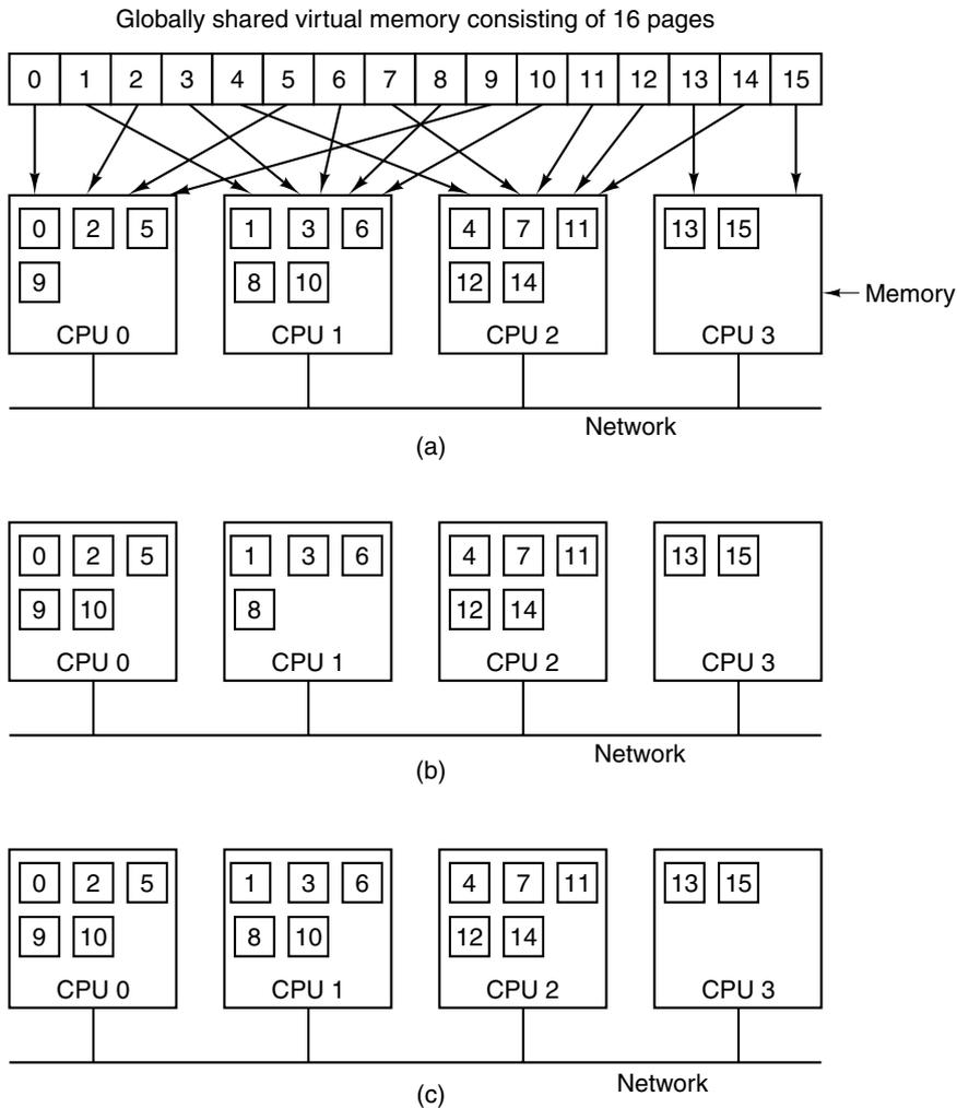
**Figure 8-44.** A virtual address space consisting of 16 pages spread over four nodes of a multicomputer. (a) The initial situation. (b) After CPU 0 references page 10. (c) After CPU 1 references page 10, here assumed to be a read-only page.
