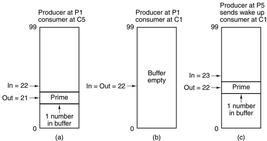
**Figure 6-26.** Failure of the producer-consumer communication mechanism.
