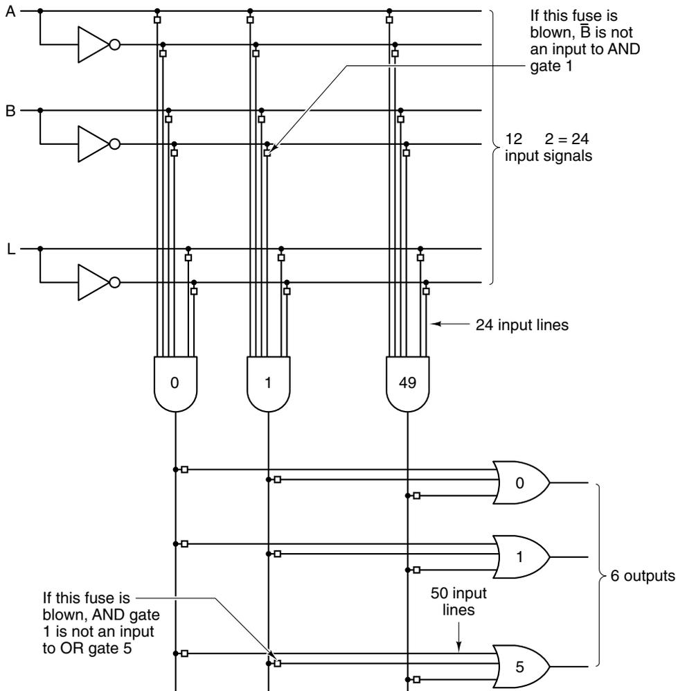
**Figure 3-15.** A 12-input, 6-output programmable logic array. The little squares represent fuses that can be burned out to determine the function to be computed. The fuses are arranged in two matrices: the upper one for the AND gates and the lower one for the OR gates.
