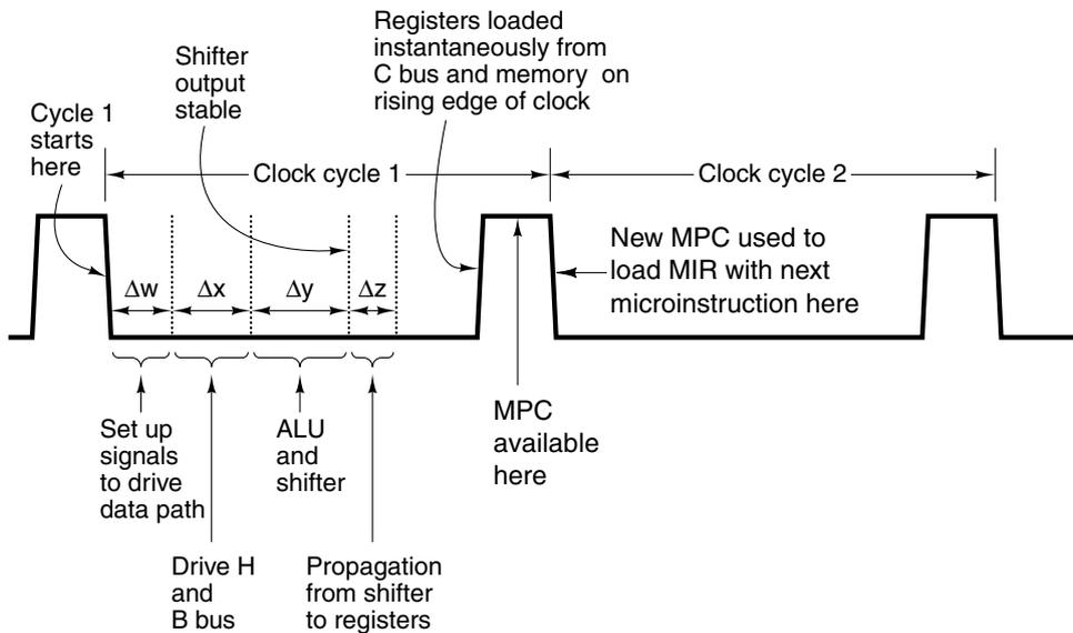
**Figure 4-3.** Timing diagram of one data path cycle.
