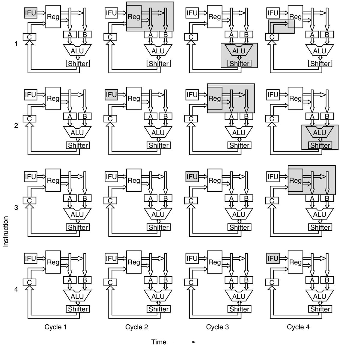
**Figure 4-34.** Graphical illustration of how a pipeline works.
