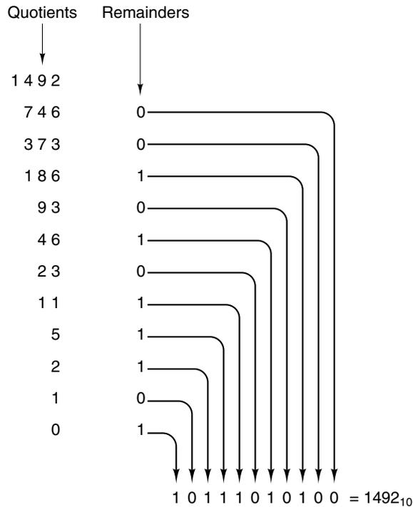
**Figure A-5.** Conversion of the decimal number 1492 to binary by successive halving, starting at the top and working downward. For example, 93 divided by 2 yields a quotient of 46 and a remainder of 1, written on the line below it.
