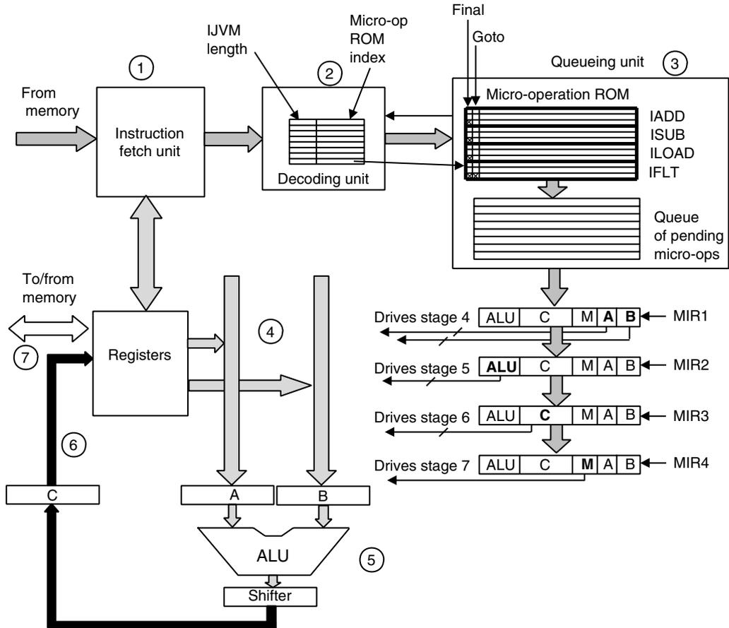
Figure 4-35. The main components of the Mic-4.
