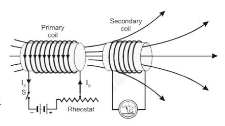
Let the flux passing through each loop of secondary is equal to  $\phi_s$ . Net flux passing through  $N_s$  loops =  $N_s \phi_s$  where  $N_s$  is the number of turns in the secondary coil.
