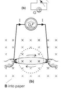
when the area is no longer changing. If the distorted coil is brought to its original circular shape thereby increasing the area, an oppositely directed current is induced which lasts as long as the area is changing.
