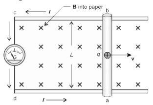
When the rod moves, a charge q within the rod also moves with the same velocity  $\overrightarrow{v}$  in the magnetic field  $\overrightarrow{B}$  and experiences a force given by
