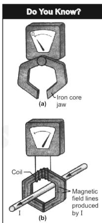
An induction ammeter with its iron-core jaw (a) open and (b) closed around a wire carrying an alternating current I. Some of the magnetic field lines that encircle the wire are routed through the coil by the iron core and lead to an induced emf. The meter detects the emf and is calibrated to display the amount of current in the wire.
