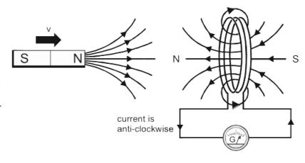
According to Lenz's law the "push" of the magnet is the "change" that produces the induced current, and the current acts to oppose the push. On the other hand if we pull the magnet away from the coil the induced current will oppose the "pull" by creating a south pole on the face of coil towards the bar magnet.
