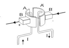
output from BB' remains in the same direction, although the current is not constant in magnitude. The curve of the current is shown in figure.
