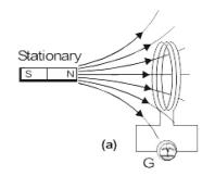
the coil, a current appears in it figure (b). As the magnet is moved, the magnetic flux through the coil changes, and this changing flux produces the induced current in the coil. When the magnet moves away from the coil, a current is again induced but now in opposite direction. The current would also be induced if the magnets were held stationary and the coil is moved.
