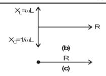
$$\begin{split} X_L &= X_C \\ \omega L &= \frac{1}{\omega C} \\ \omega^2 &= \frac{1}{LC} \\ \omega &= \frac{1}{\sqrt{LC}} \\ 2\pi f_r &= \frac{1}{\sqrt{LC}} \\ f_r &= \frac{1}{2\pi\sqrt{LC}} \end{split}$$
