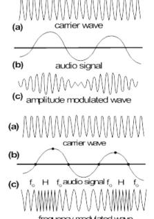
The F.M. transmission frequencies are much higher and ranges between 88 MHz to 108 MHz. F.M. radio waves are affected less by electrical interference than A.M. radio waves and hence, provide a higher quality transmission of sound. However, they have a shorter range than A.M. waves and are less able to travel around obstacles such as hills and large buildings.
