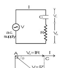
This shows that current leads the applied voltage by an angle ' $\theta$ '.
