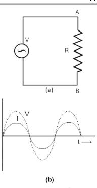
It is very important to noted that this equation holds only when current and voltage are in phase.
