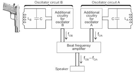
are the same and hence the resonance frequency of the two circuits is also same. When the inductor B; called the search coil comes near a metal object, its inductance L<sub>B</sub> decreases and corresponding oscillator frequency increases and thus a beat note is heard in the attached speaker. Such detectors are extensively used not only for various security checks but also to locate buried metal objects.
