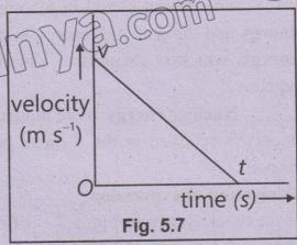
Suppose a body of mass m is moving with velocity v. An opposing force F is acting on the body through a distance S brings it to rest. Then,
