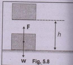
The applied force necessary to lift the block with constant velocity is equal to weight w of the block and since w = mg, therefore, potential energy of the block at height h becomes,
