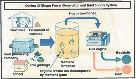
Fig: 27.16 Biogas production mechanism.
