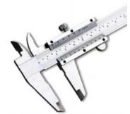
**Fig 1.14 Vernier Calipers**
