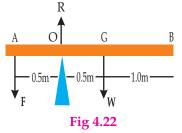
A uniform rod of length 2.0m is placed on a wedge at 0.5m from its one end (Fig4.22). A force of 150N is applied at one of its ends near the wedge to keep it horizontal. Find the weight of the rod and the reaction of the wedge.
