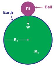
**Fig 6.5** Weight of a ball is equal to the gravitational force between the ball and the Earth.
