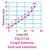
Table 5.1 shows how a spring stretches as the load on it increases. Dependance of extension on load, shown in Fig 5.3 (c).
