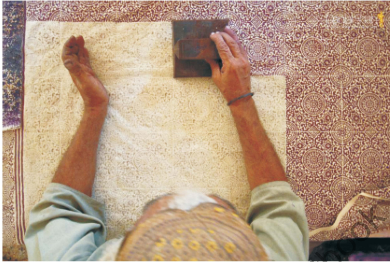
Figure 8.19 Printing of Ajrak with wooden blocks
