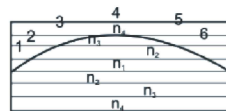
Fig. Light propagation within a hypothetical multi layer fibre
