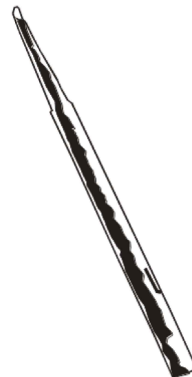
Fig. (b) A precision diamond scalpel for use in eye surgery. The illumination is obtained by light passing through a fibre optic light guide.
