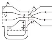
As the cross sectional area  $A_2$  is small as compared to the area  $A_1$ , then from equation of continuity  $V_1 = (A_2/A_1) V_2$ , will be small as compared to  $V_2$ . Thus for flow from a large pipe to a small pipe we can neglect  $V_1$  on the right hand side of equation, hence,
