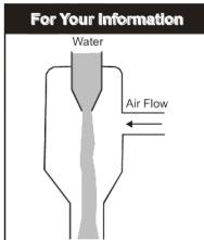
A filter pump has a constriction in the centre, so that a jet of water from the tap flows faster here. This cause a drop in pressure near it and air, therefore, flows in from the side tube. The air and water together are expelled through the lower part of the pump.
