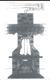
A chimney works best when it is tall and exposed to air currents, which reduces the pressure at the top and force the upward flow of smoke.
