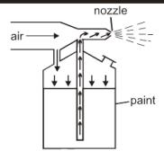
A stream of air passing over a tube dipped in a liquid will cause the liquid to rise in the tube as shown. This effect is used in perfume bottles and paint sprayers.
