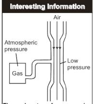
The carburetor of a car engine uses a Venturi duct to feed the correct mix of air and petrol to the cylinders. Air is drawn through the duct and along a pipe to the cylinders. A tiny inlet at the side of duct is fed with petrol. The air through the duct moves very fast. creating low pressure in the duct, which draws petrol vapour into the air stream.
