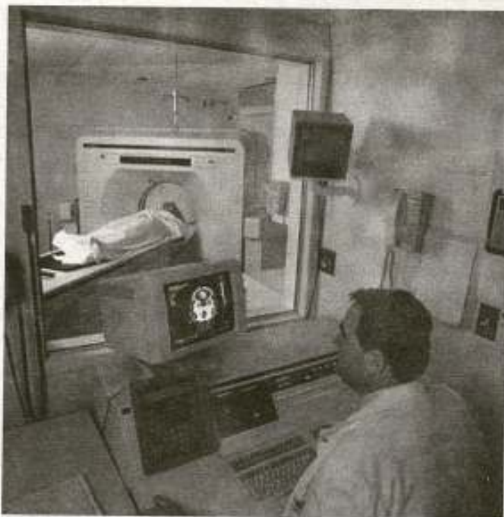
Figure 4.7: Computed axial topography (CAT) still uses X-rays to see inside the body. But instead of using a single beam, a CAT scanner takes many X-rays around the body. The scanner's computer then builds up pictures of a 'slice' through the body and combines them to give a 3D image. Scientists used CAT to carry out the first detailed studies of the brain, before even more powerful techniques were developed.
