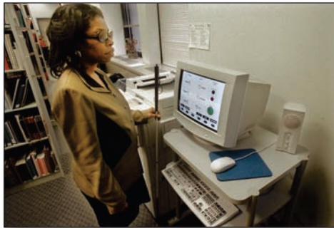
Regina Genwright talks to a voice-activated copier at the American Foundation for the Blind. The copier has a Braille keyboard and is wheelchair-accessible height. Equipment like this can help employers make reasonable accommodation for their disabled employees.
